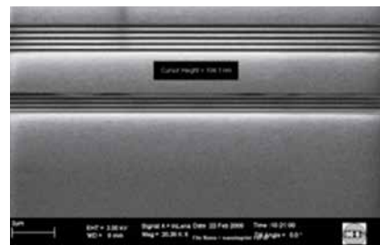
UV-NIL: 50 nm, 70 nm lines and spaces imprinted with MJB4 Mask Aligner
