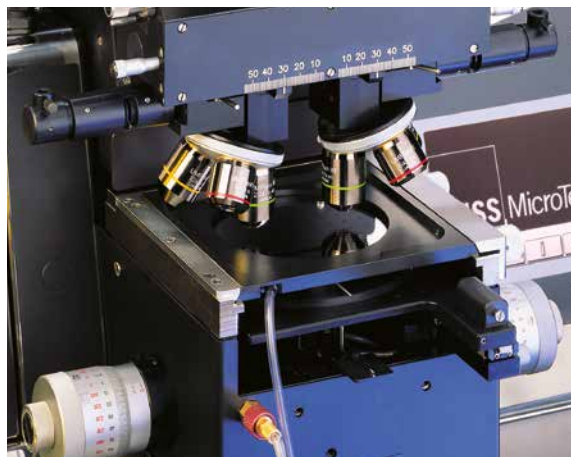
Optical system of a SUSS MJB4 Mask Aligner
