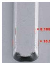
Printed resist profile with measured line width
