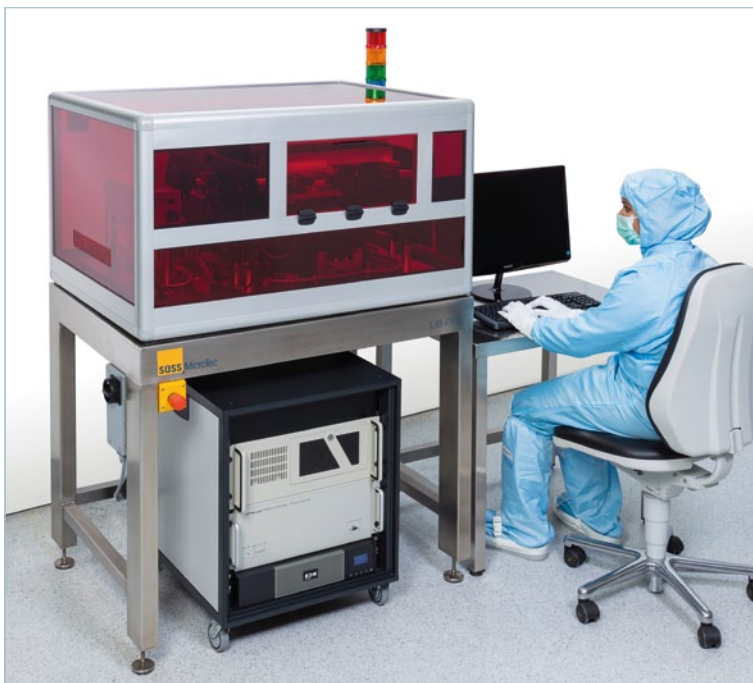
Figure 2 The SUSS LI8 Pro model: The Write Unit contains the laser source(s), the chuck for the different substrates, and the XYZ stages that move the substrate under the focused laser beam. A rack cabinet contains the Control Unit
